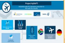
The project entails ~ 500MW of wind and solar electricity supplying electricity to a 200 MW electrolyser that will produce ~20 ktpa of green hydrogen. The green hydrogen will be combined with industrial carbon dioxide in Sasol's existing Fischer Tropsch facilities to produce ~50 kt/a of PtL-Kero type Sustainable Aviation Fuel (SAF).
