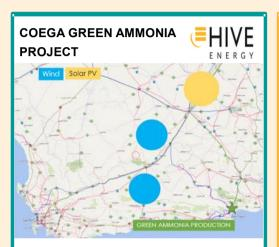
The proposed Hive Hydrogen South Africa project entails the development of Solar PV (1430MW) and Wind (2108MW) facilities will be wheeled across the Eskom network to drive which will supply 1120MW of Electrolyser plant to produce 1,000 ktpa of Green Ammonia. The project is located in the Coega port/SEZ area.
