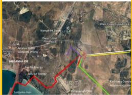
The proposed Assegai Project entails a 1000MW Natural Gas to Power Plant with LNG Storage and Regasification, Overhead Electricity Transmission, and Associated Infrastructure. The project is located within the Bessansklip Industrial Zone in Saldanha Bay.
